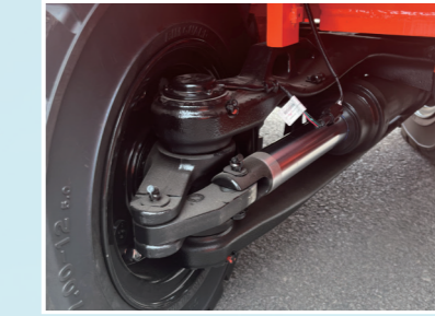
Cast Internal Combustion Forklift Steering Axle.
