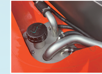
Convenient hydraulic oil level check.
